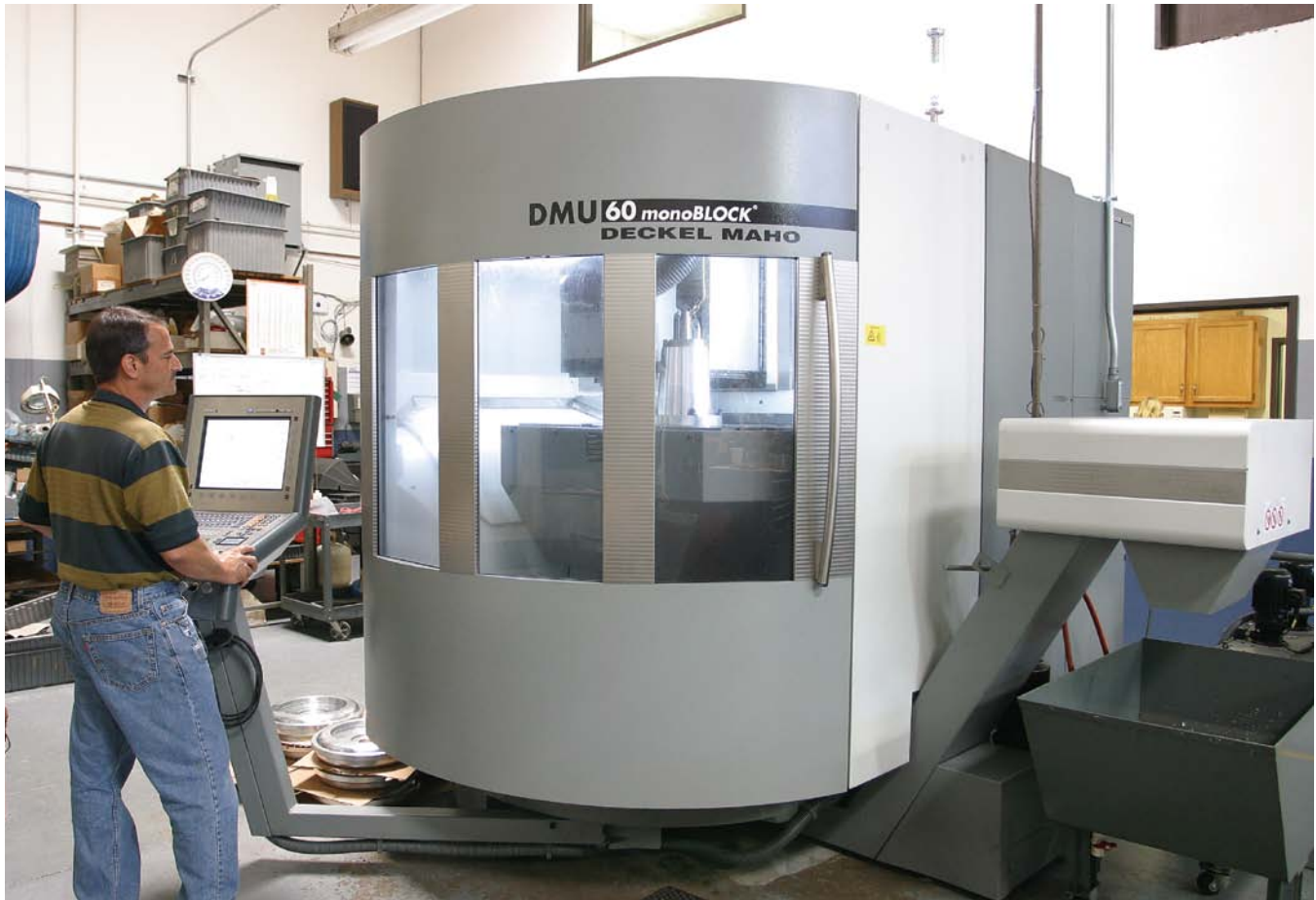
Polynetics' acting president Robert Pernice programs his new DMU 60 monoBLOCK 5-axis machining center. The machine has a work area of 28.7" x 22" x 22" With it's 18,000 rpm spindle the machine delivers rapids up to 2,000 ipm and cutting speeds up to the rapids rate. The controller is a Heidenhain system that Pernice programs with Open Mind Hypermill software.
